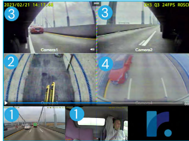
Six camera view on RoscoLive (DV6 in-cab view + exterior windshield view, two side camera views, interior cargo view, backup camera view)
